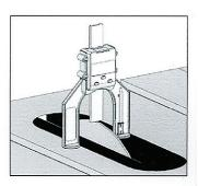
3. Install the plunger and zero the gauge for measuring depths as shown below.
