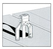
2. Set your router bit or saw blades to the desired position as shown.
